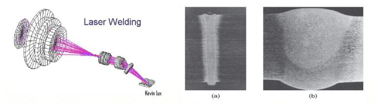
Comparison of the sizes of weld beads: (a) laser-beam or electron-beam welding and (b) tungsten arc welding.
