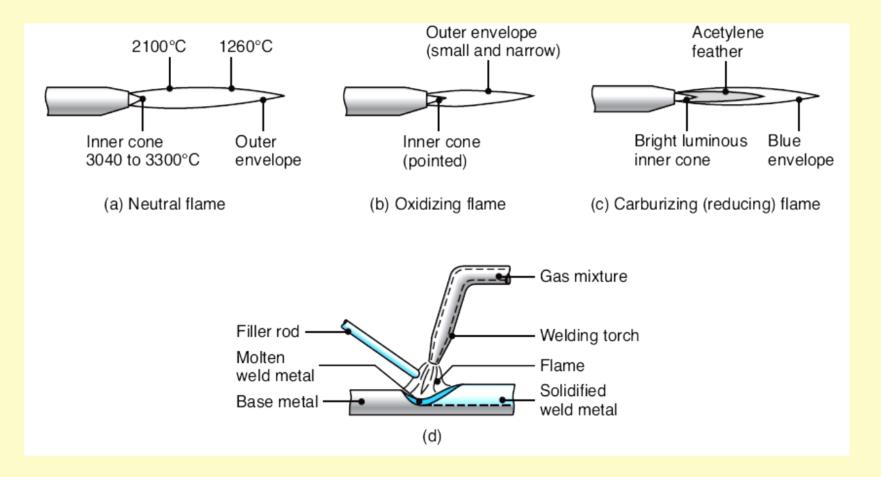
The gas mixture in (a) is basically equal volumes of oxygen and acetylene. (d) The principle of the oxy fuel–gas welding process.
