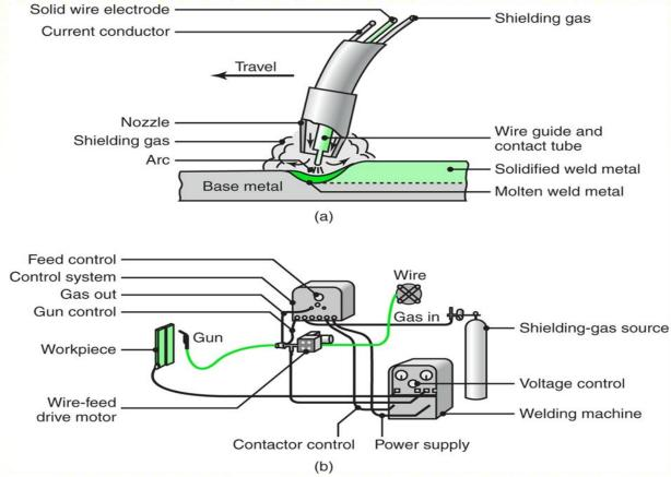
(a) Schematic illustration of the gas metal-arc welding process, formerly known as MIG (for metal inert-gas) welding. (b) Basic equipment used in gas metal-arc welding operations.
