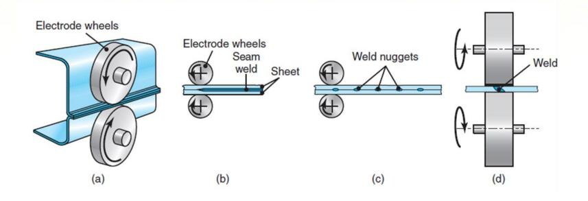
(a) Seam-welding process in which rotating rolls act as electrodes. (b) Overlapping spots in a seam weld. (c) Roll spot welds and (d) Mash seam welding.
