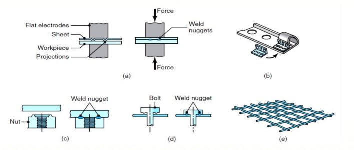
(a) Schematic illustration of resistance projection welding. (b) A welded bracket. (c) and (d) Projection welding of nuts or threaded bosses and studs.
