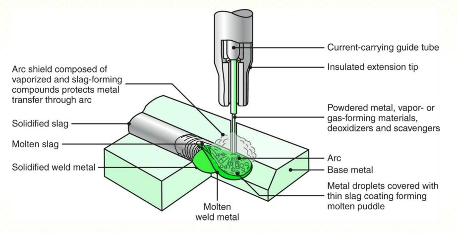
Schematic illustration of the flux-cored arc-welding process. This operation is similar to gas metal-arc welding
