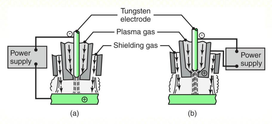
Two types of plasma-arc welding processes: (a) transferred and (b) non-transferred. Deep and narrow welds can be made by these processes at high welding speeds.
