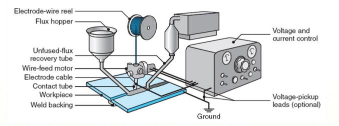
Schematic illustration of the submerged-arc welding process and equipment. The un fused flux is recovered and reused.
