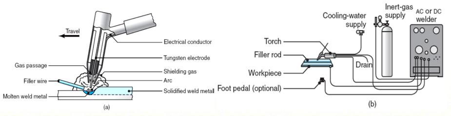
(a) The gas tungsten-arc welding process, formerly known as TIG (for tungsten-inertgas) welding. (b) Equipment for gas tungsten-arc welding operations.
