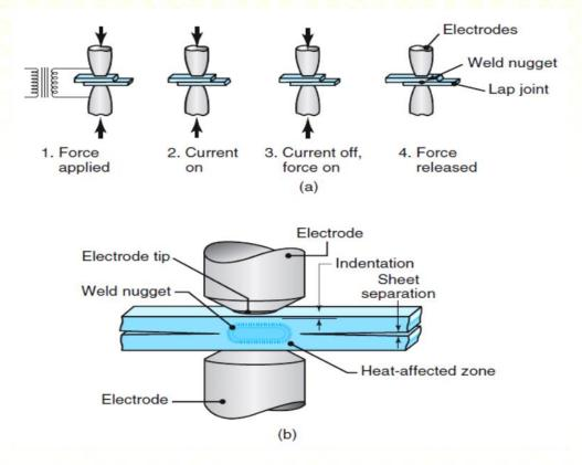
Sequence of events in resistance spot welding. (b) Cross section of a spot weld, showing the weld nugget and the indentation of the electrode on the sheet surfaces. This is one of the most commonly used processes in sheet-metal fabrication and in automotive body assembly.
