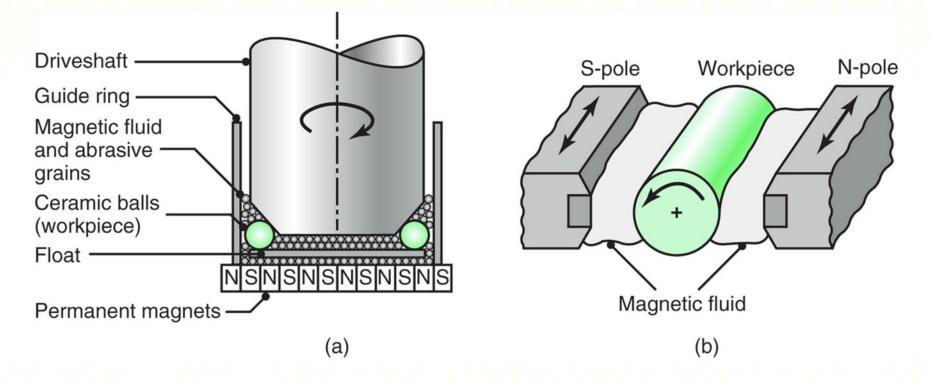
(a) Magnetic-float polishing of ceramic balls. (b) Magnetic-field-assisted polishing of rollers.
