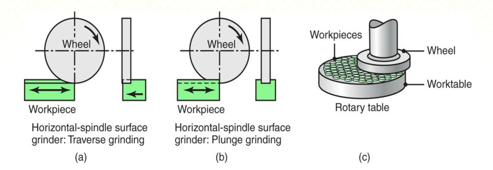
(a) Traverse grinding with a horizontal-spindle surface grinder. (b) Plunge grinding with a horizontal spindle surface grinder, producing a groove in the work piece. (c) A vertical-spindle rotary table grinder (also known as the *Blanchard* type).
