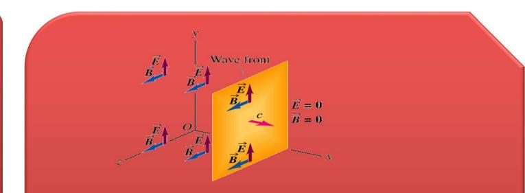
An electromagnetic wave front. The plane representing the wave front (yellow) moves to the right with speed c.
