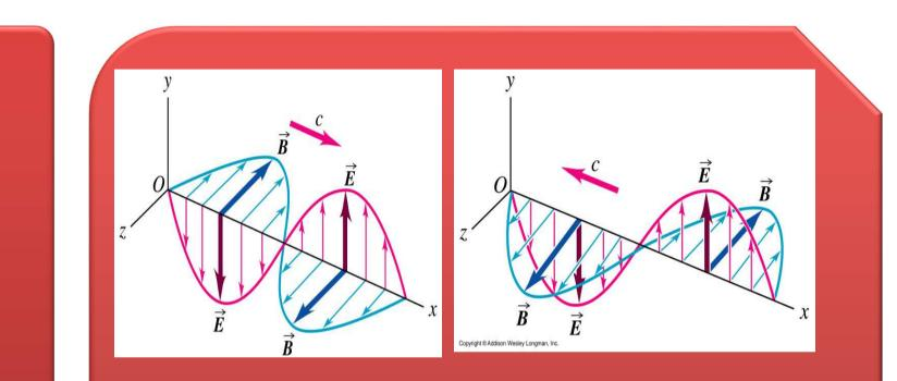
Representation of the electric and magnetic fields in a propagating wave. One wavelength is shown at time t = 0.
