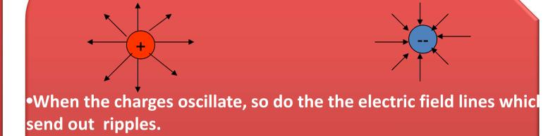
•The ripples can be created in the directions orthogonal to the direction of oscillation (transverse wave).
