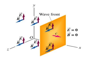
An electromagnetic wave front. The plane representing the wave front (yellow) moves to the right with speed c.
