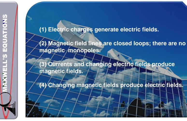
From Maxwell's equations one can derive another equation which has the form of a "wave equation".
