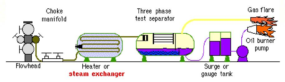
The HEATER (or STEAM EXCHANGER) is used to raise the effluent temperature above hydrate formation point, to reduce viscosity (heavy crude oil) or to break the emulsion.
