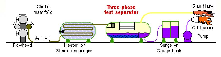
The SEPARATOR is the main surface testing piece of equipment. It separates the three phases of the effluent which can then be metered and sampled individually.
