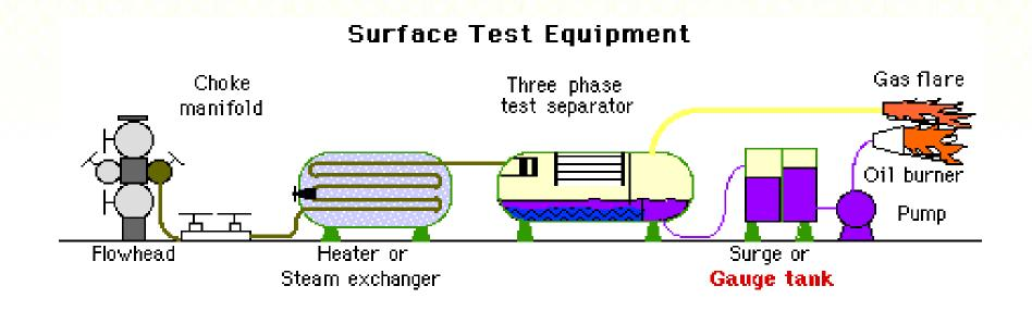
The ATMOSPHERIC GAUGE TANK and the SURGE TANK are used to calibrate the separator liquid flow measurement, and to measure the flow in case of low oil flow rates.
