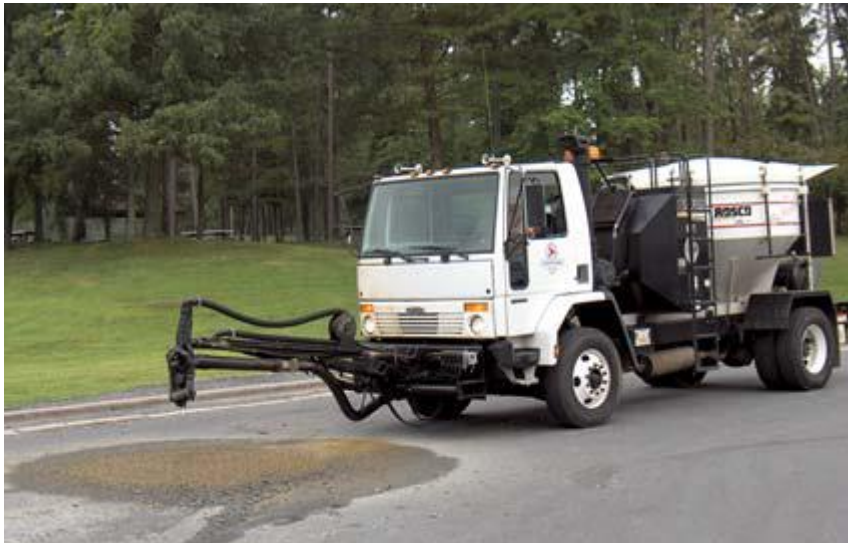
Teleoperated pothole patching robot
