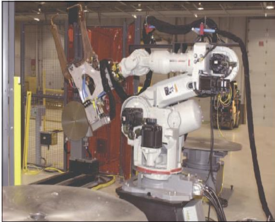
Motoman UP200 robot spot welds large agricultural equipment assemblies
