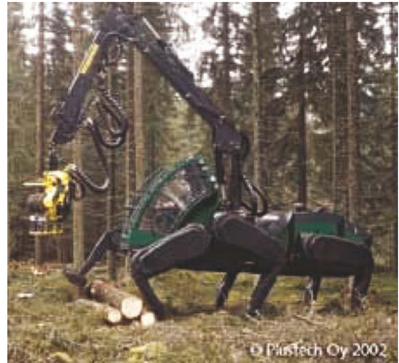
Walking forest harvester prototype by Plustech Ltd., today part of John Deere
