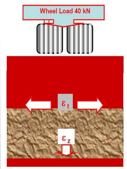
Bituminous Wearing Course Durability, Safety (Skid Resistance, Smoothness), Strength
