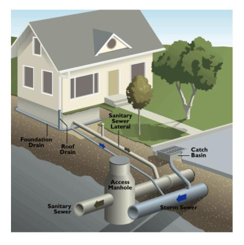
Sewer **Pipes** or channels to convey sewage to sewage treatment plant
