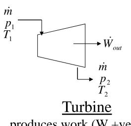
produces work (W +ve) from expansion of fluid ( $\Delta P$  -ve)
