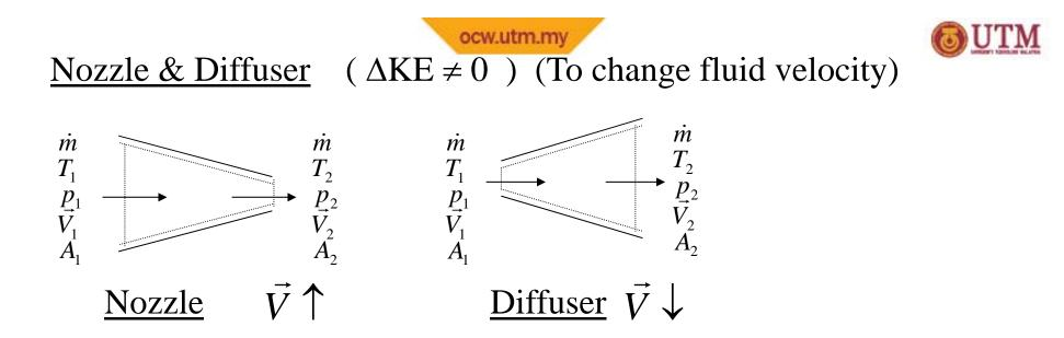
$\frac{\text{Assumptions}}{\text{Const. volume}} \rightarrow w_{\text{B}} = 0$ No other work  $\int w_{\text{CV}} = 0$   $\text{Small difference in height} \rightarrow \Delta \text{pe} = 0$   $\dot{Q} - \dot{W} = \sum_{out} \dot{m}(h + ke + pe) - \sum_{in} \dot{m}(h + ke + pe)$ 1 inlet / 1 outlet  $q - \dot{W} = \Delta h + \Delta ke + \Delta \dot{p}e \qquad q = \Delta h + \Delta ke$
