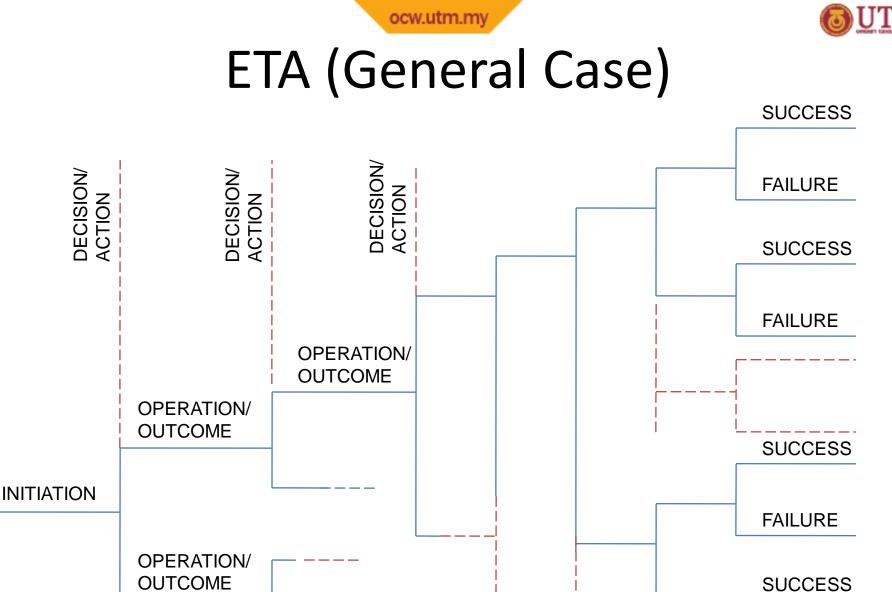
Portray all credible system operating permutations Trace each path to eventual success or failure FAILURE
