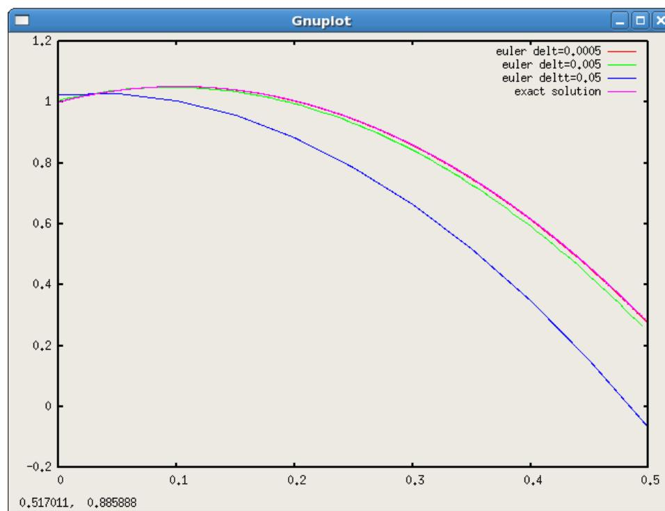
The **smaller** the **delt** the closer the curve to the **exact solution**.
