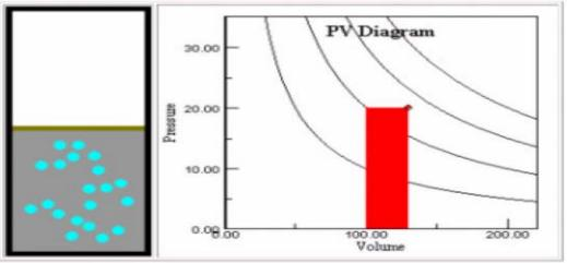
The work done by the system: the pressure multiplied by the change in volume
