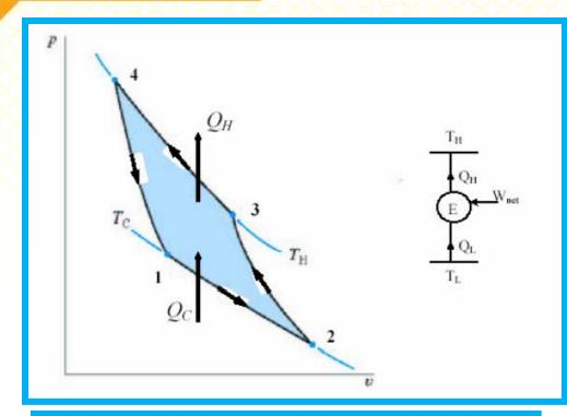
Q<sub>C</sub>: heat is removed from cold reservoir
