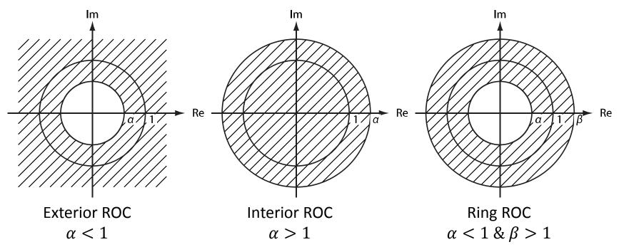
For FIR system, ROC is the entire z-plane except at 0 and ∞. Thus, unit circle is always inside the ROC. This means that, FIR system is always stable.
